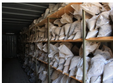
Figure 8: Reverse-circulation drill chip samples stored on site at La Corona de Cobre.
